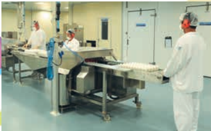
The production of the vaccine is based on the use of fertilized chicken eggs.
