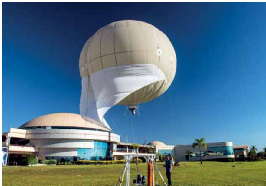
Positioned up to 200 meters above the ground, the balloons manufactured by Altave are 3 to 7 meters in diameter
