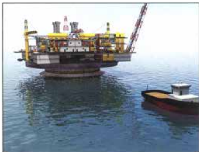
Monocolumn keeps the platform stable
