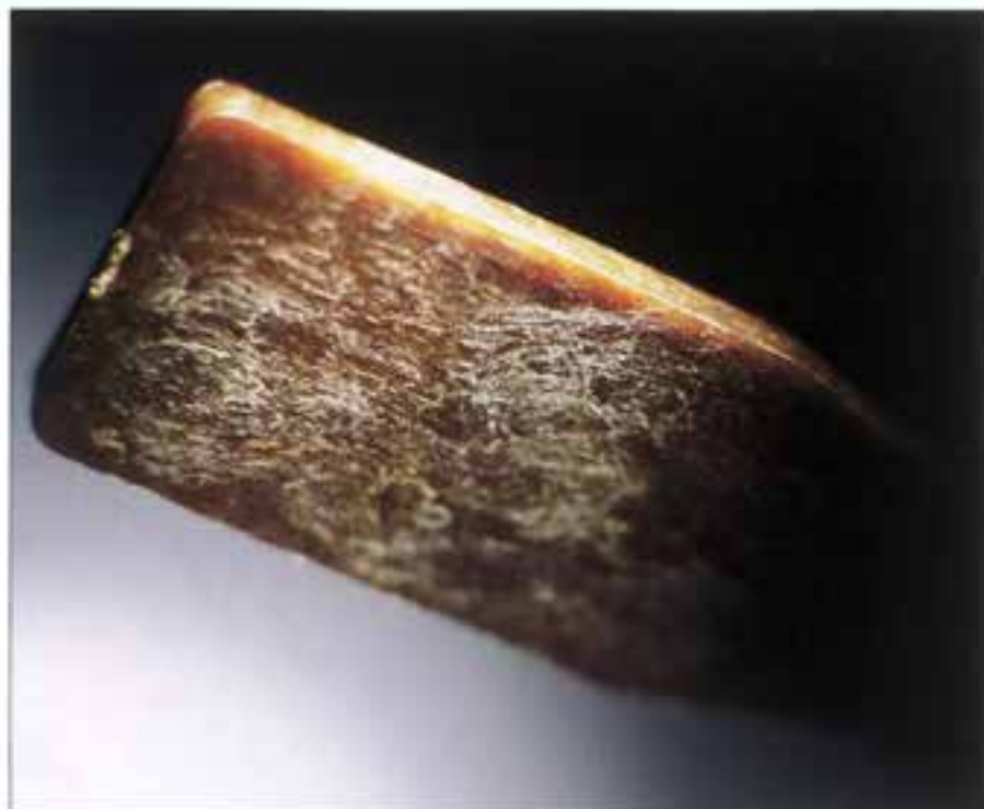
The Curauá: fibrous leaves and a fruit smaller than the pineapple. Above, part of a composite used in the roofing of cars
