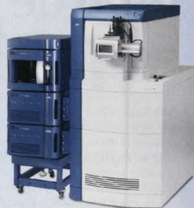
Sistema LC/MS/MS composto de nanoAcquity™ e detector Q-TOF Premier
