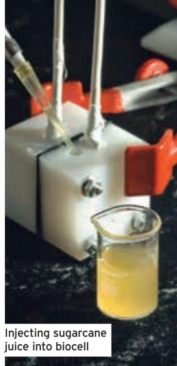
Injecting sugarcane juice into biocell
