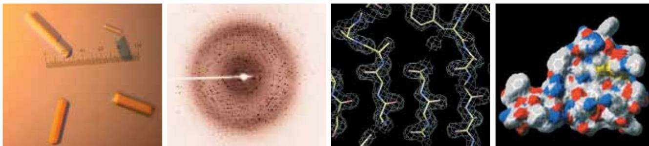
Stages of identification of the spatial structure of an anti-coagulant, the inhibitor of factor XII: from left to right, crystals seen under a magnifying glass (scale, 100 = 1 mm) and by X-ray diffraction before atom by atom reconstitution of the molecule
