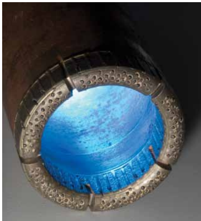
Drill tip coated with synthetic diamond for oil exploration
