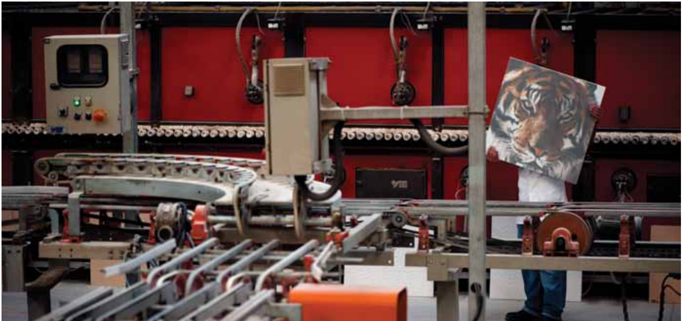
At the Villagres company, digital printing technology reproduces the photo of a tiger on a ceramic floor tile
