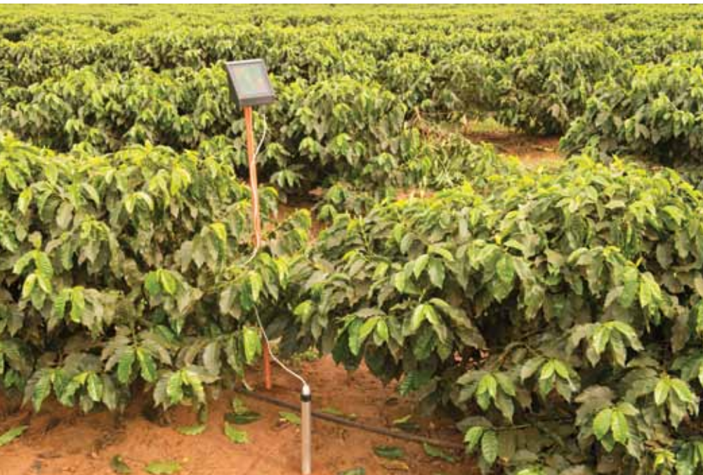
1 Moisture sensor among coffee plants developed jointly by Unesp, CDMF and Sencer
