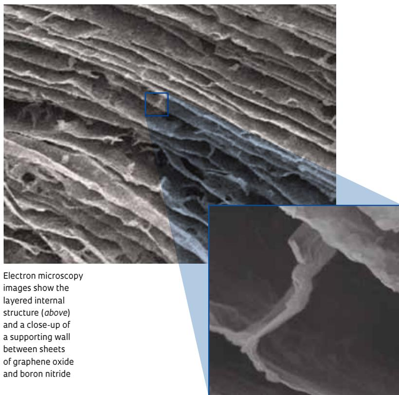
Electron microscopy images show the layered internal structure (above) and a close-up of a supporting wall between sheets of graphene oxide and boron nitride
