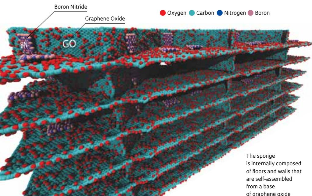
The sponge is internally composed of floors and walls that are self-assembled from a base of graphene oxide layers reinforced with sheets of boron nitride
