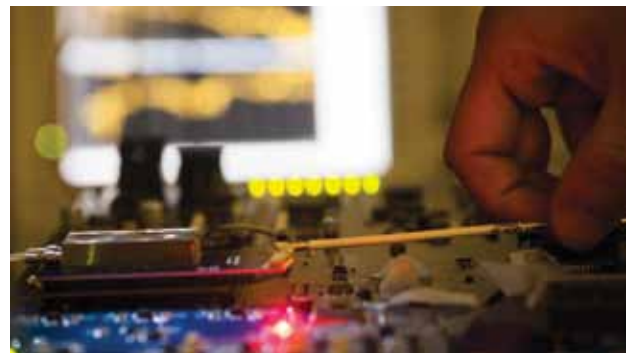
Fiber optic alignment (above) and close-ups of the company's high-speed optical transmitter, called TOSA
