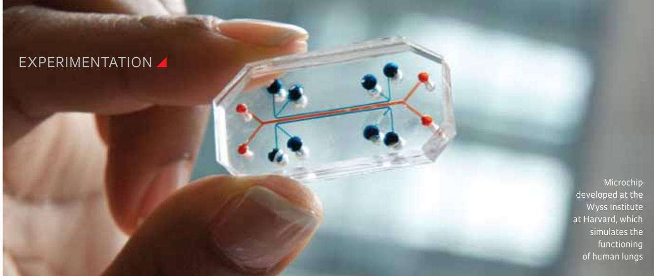
Microchip developed at the Wyss Institute at Harvard, which simulates the functioning of human lungs
