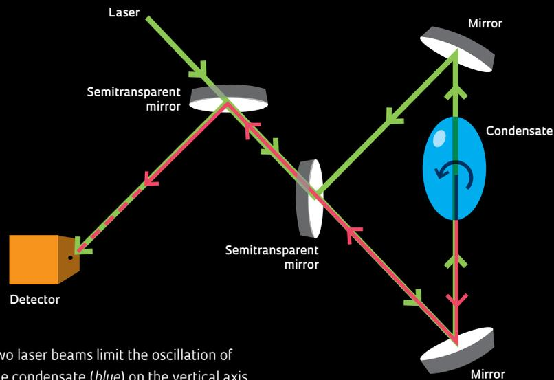
Two laser beams limit the oscillation of the condensate (blue) on the vertical axis, and a third laser beam (green) monitors its displacement, which is affected by gravity. A detector reads the light (in red) that results from the interaction of the condensate with the green laser
