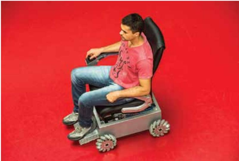
Easy maneuverability using a wheelchair that moves in every direction (above). With four uniform omnidirectional wheels, the device has small rollers that allow movement in any direction (left)
