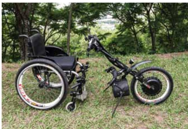
*Kit Livre:* accessory that consists of a wheel, handlebars and rechargeable electric motor that can be attached to a manual wheelchair
