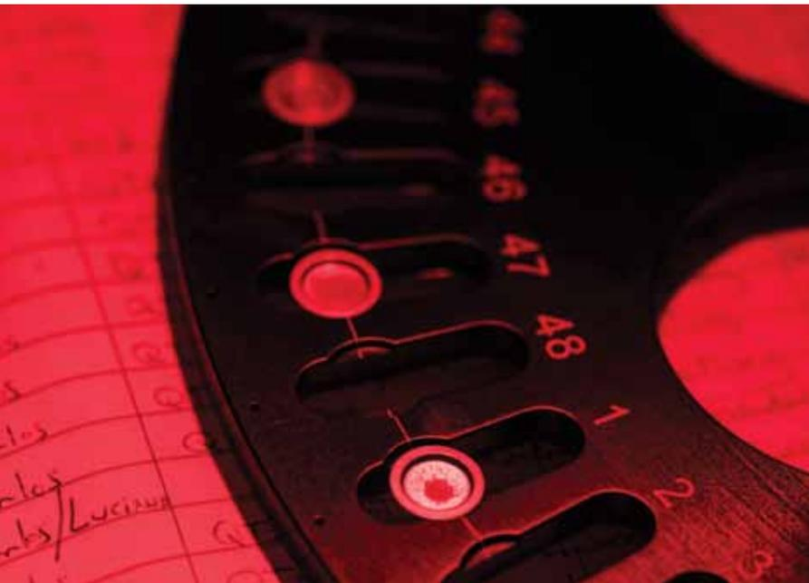
In a laboratory illuminated only by red light, one can find out when samples of sediment last received sunlight
