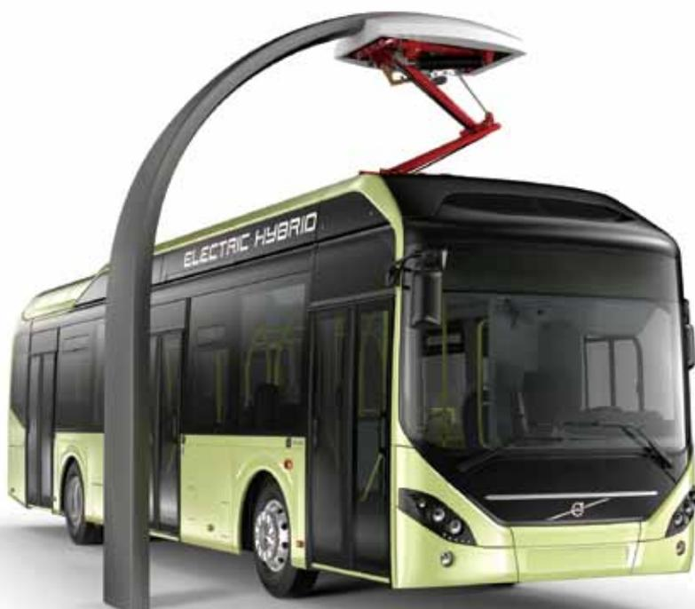
Option in Europe: quick recharging of batteries at points of passenger entry or departure
