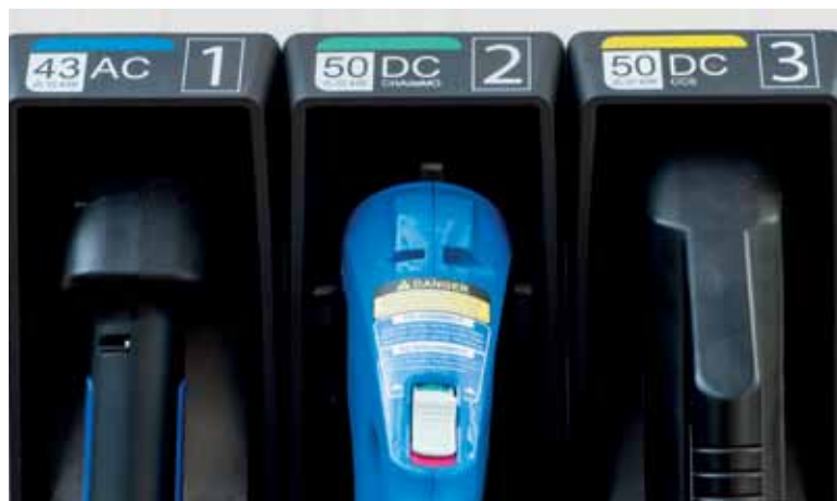
Different types of rapid recharge plugs and connectors at an electric vehicle recharging station
