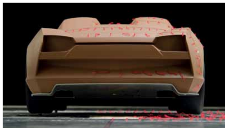
Small-scale model of the Electric Dreams supercar: tests are conducted in a wind tunnel
