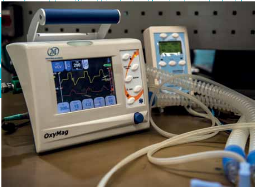
OxyMag is a portable respirator for use in ambulances with ICU equipment
