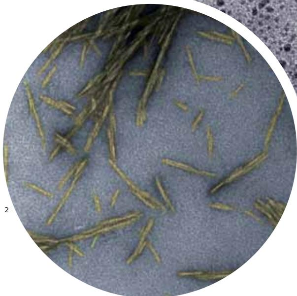
Nanocrystals used to reinforce cement
