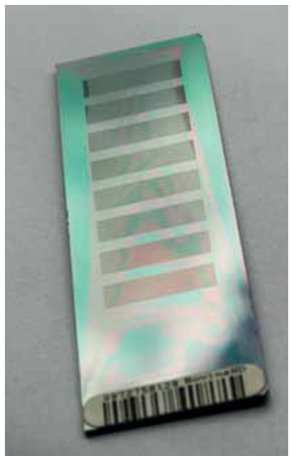
The bovine DNA chip is a blade with sensors used to determine familial relationships within a group of animals, as well as to identify genetic defects
