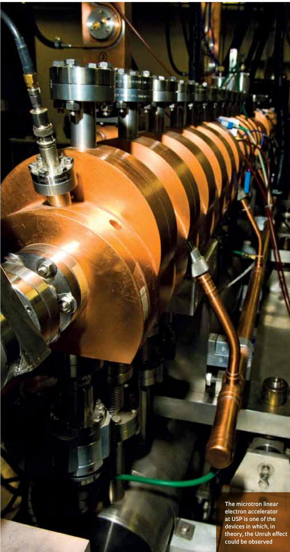
The microtron linear electron accelerator at USP is one of the devices in which, in theory, the Unruh effect could be observed
