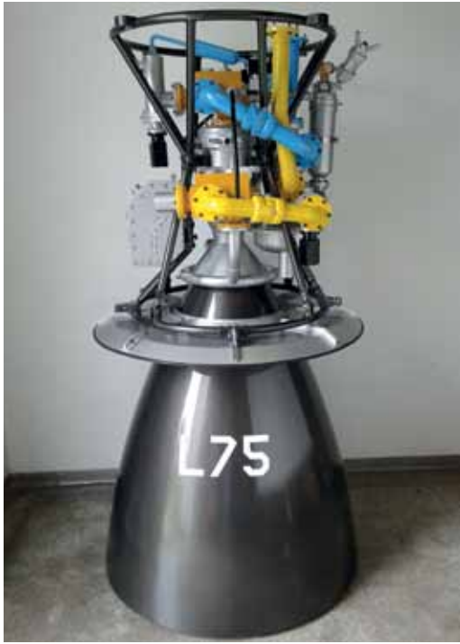
Model of the L75 rocket developed at IAE, which uses ethanol and liquid oxygen
