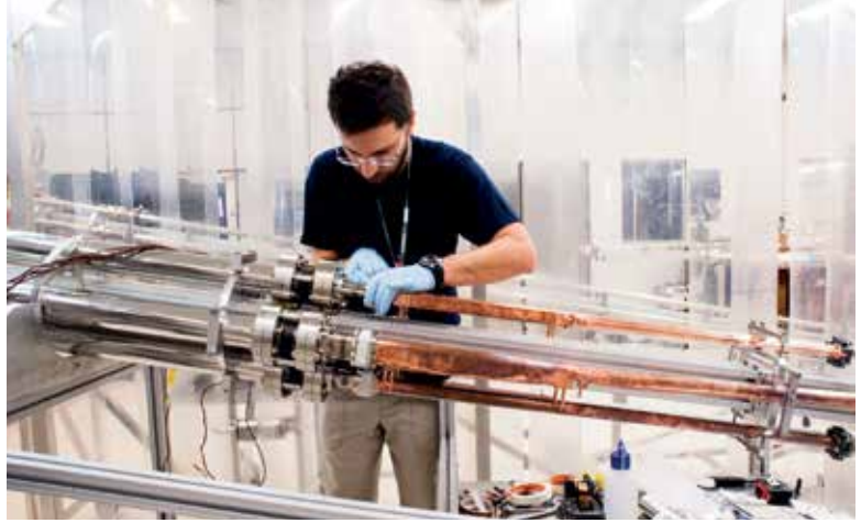
Engineer Rafael Seraphim tests the vacuum system of the chambers that will propel the electrons. Left, quadrupole magnets, one of the components of the storage ring
