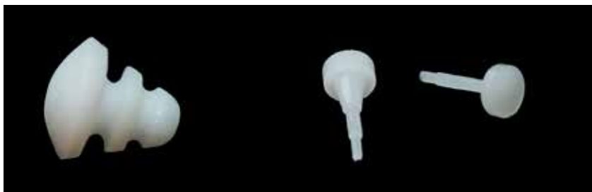
Bioactive glass ceramics: an eye implant ( left ) and middle-ear ossicles
