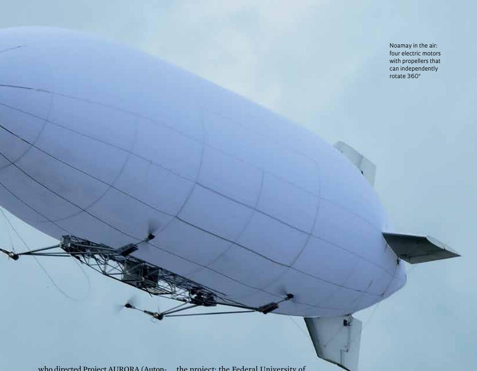
Noamay in the air: four electric motors with propellers that can independently rotate 360°
