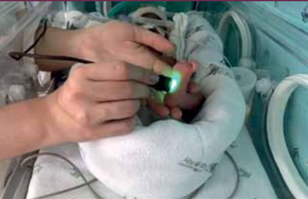
The UFMG researcher uses a device that measures the light reflected by skin to estimate the gestational age of a baby
