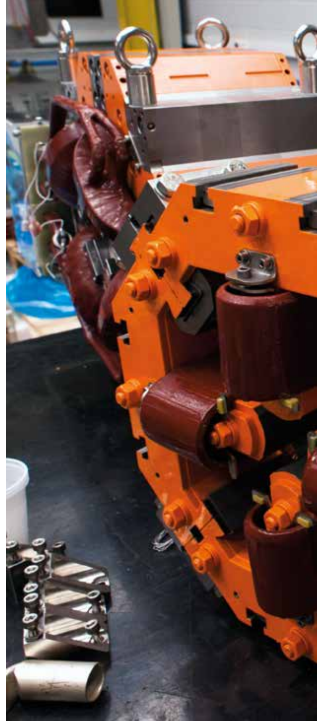
The electromagnets during magnetic characterization testing on the Sirius synchrotron light source
