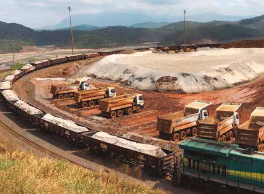
Reused sand from iron mine tailings from Vale's Cauê mine in Itabira, Minas Gerais state
