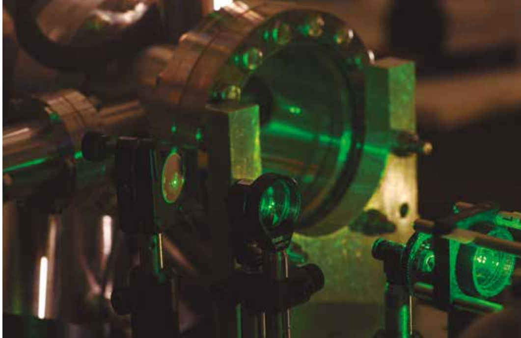
The rear window of the chamber used to allow the passage of light for measurement
