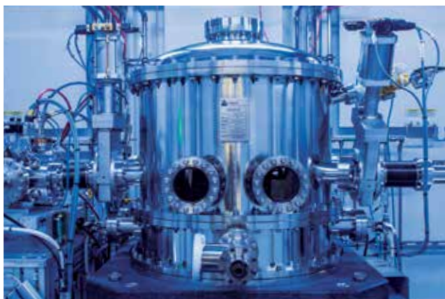
Monochromator: part of the CARNAÚBA beamline at Sirius, where the study was carried out
