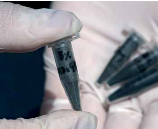
Samples of bioglass with different compositions of magnetic material
