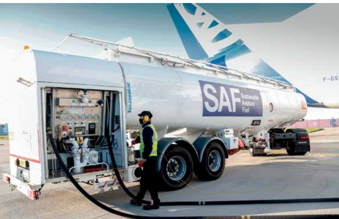
Aircraft produced by the European manufacturer Airbus is fueled with aviation biofuel
