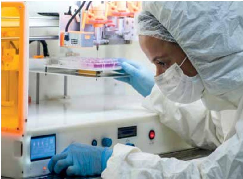
Ana Luiza Millás of 3DBS operates a bioprinter; in a close-up, the syringe deposits the cell solution into the compartments of a tray
