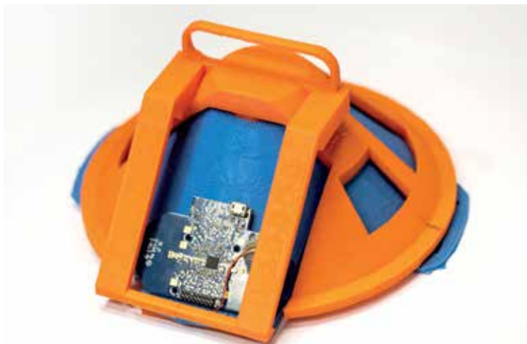
Prototype of the microwave imaging system designed by USP and IFSP
